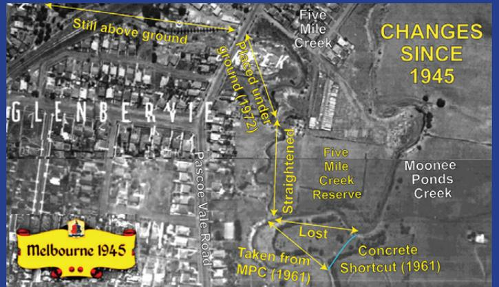
The lower reaches of the creek were also undergoing many changes - I have marked them on this Melbourne 1945 aerial view. The section just east of Pascoe Vale Road was placed underground in 1972 - by the MMBW, but at the expense of the landowner. The final section of the present day Five Mile Creek was originally part of the Moonee Ponds Creek. It was stranded when the concrete shortcut was created in 1961!
